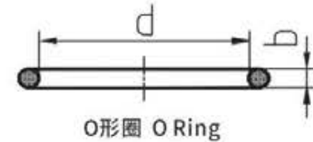
公制外螺纹可调向柱端用O形圈 For Metric Male Adjustable Stud End O-ring
